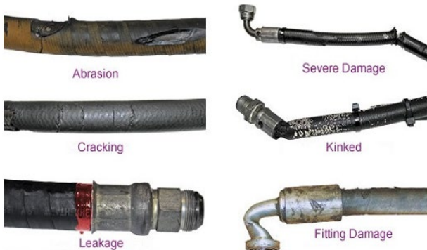
Fig. 2. Examples of Damaged Hydraulic Hose
