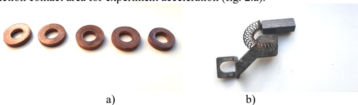
Fig. 2. Experimental testing samples: a) – new just fabricated copper samples simulating contact ring commutator: b) – real graphite alternator brush simulating itself.
