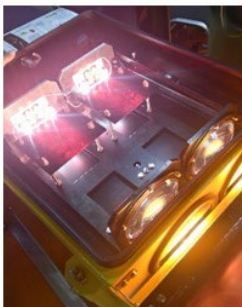
Fig. 4. Glide fire consists of six white and six red LEDs
